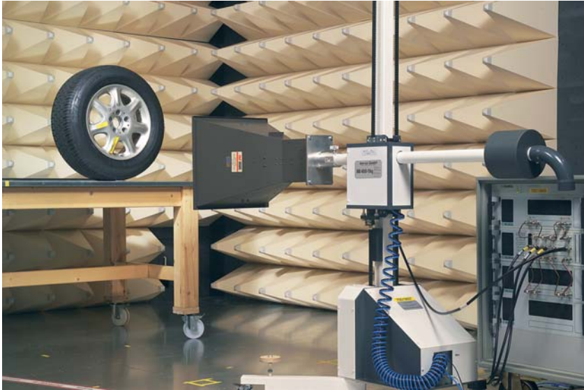
Figure 4: Radiated immunity test on a wheel electronic device
