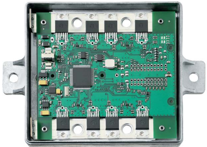
Figure 4: A view of the new ISS control unit, which can be fitted to the engine. It communicates with the drive train components via a customer-specified CAN interface, and controls the glow plugs and the heater flange
