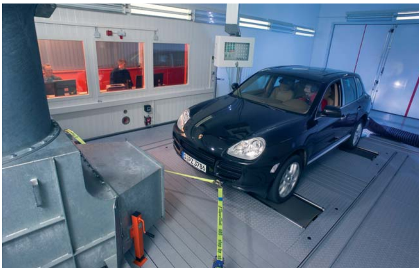
Figure 11: The new BERU cold cell with two-axle roller dynamometer
